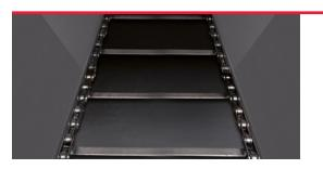
The system consists of a wide metal belt made of steel with high strength cross bars. The metal belt is driven by pinions which maintain constant traction and correct timing without sliding.
