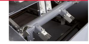
This allows material to flow continuously from the hopper to the spreading unit, breaking down any lumps and preventing them from dropping in an uncontrolled way.
