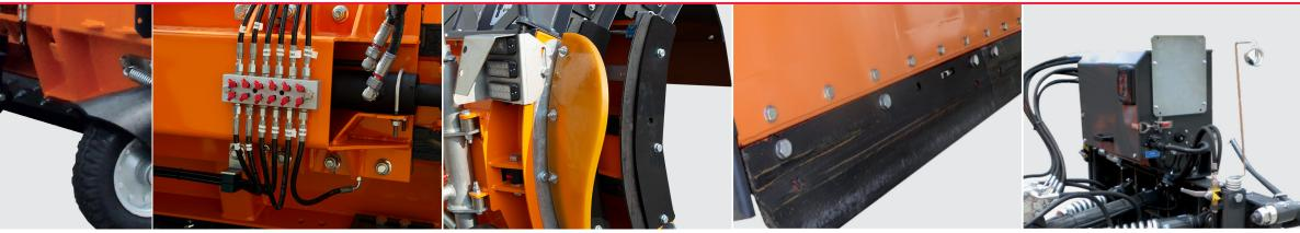
Centralized greasing system (optional) Placed in an easy accessible but and protected position, it is connected to all the lubrication points and makes maintenance work easier. LED backlighting (optional) On the left and right ends, it increases rear visibility of the snowplough.
