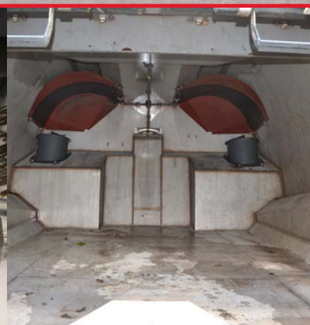
Easiclean* Easiclean option can connect to a hydrant to flush the inside of the hopper, cleaning the roof duct and behind the inlet tubes.
