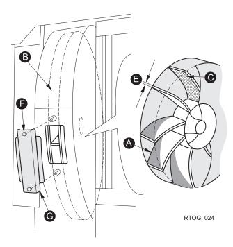
Refit the inspection plate securely after inspection / cleaning.
