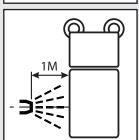
• The nozzle distance should be greater than 1 metre minimum from the panel  $\checkmark$
