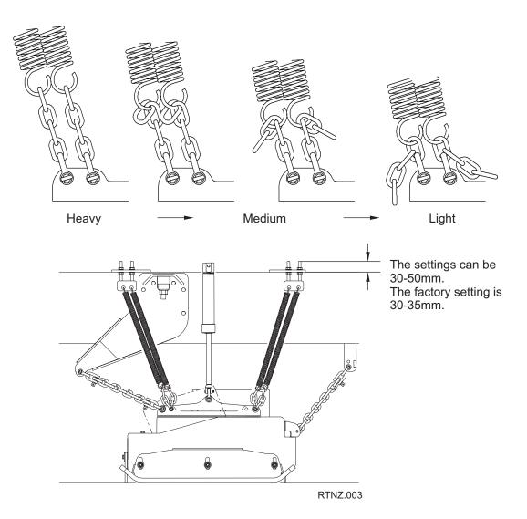
By moving the spring support upwards to 50mm you can tension the springs to fine adjustment. The initial factory setting is 30 - 35mm. Both sides on the pick-up hood should be adjusted in the same way, although subject to road camber you might want to alter these settings to suit conditions.
