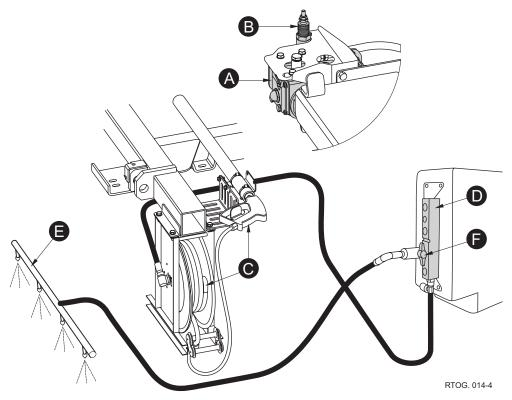
The equipment comprises a hydraulically driven high pressure water pump (A) and unloader valve (B) fitted to the subframe centre crossmember. A hand lance with 15 metres of hose on a recoiling reel (C) mounted to the subframe rear crossmember and a manifold (D) attached to the nearside water tank. An optional front spraybar (E) is available with isolating valve (F). The spraybar can be used during sweeping operations to jet wash the road prior to, or after, sweeping.
