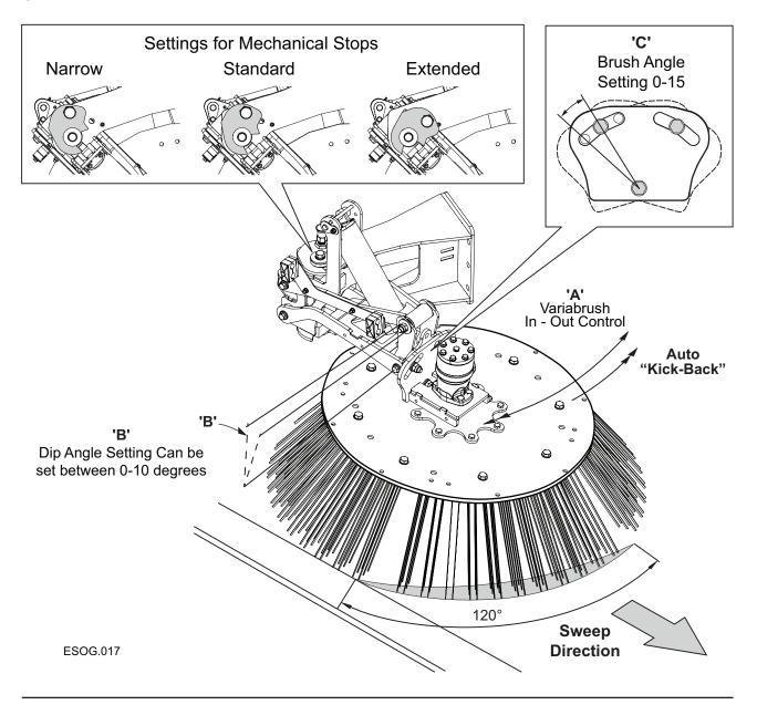
The brush angle should be set using adjustment (C) and (D) so that only about 120° of the circumference towards the front kerb is in contact with the road.
