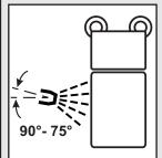
• The spray angle should be maintained between 90 and 75 degrees to the panel  $\checkmark$
