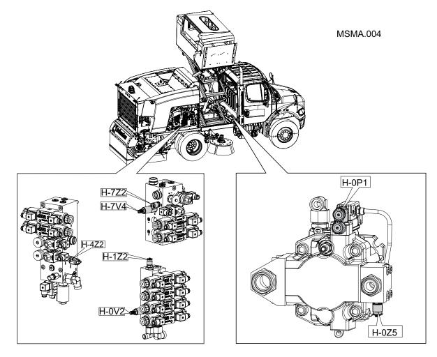
Test points are provided on the hydraulic system to carry out pressure checks.
