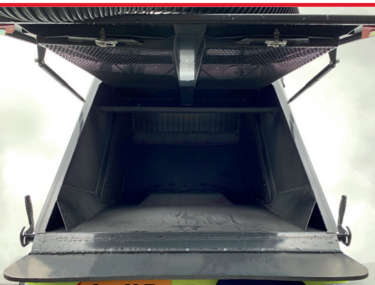
Hopper 1.8 m³, stainless-steel
