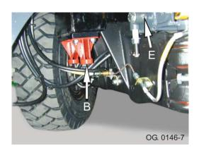
B = Jacking Point - Bottle JackE = Check Strap Pivot Grease Point (coil suspension only)
