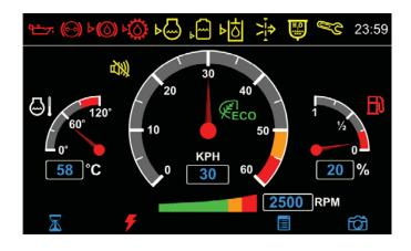
When work mode is selected (by selecting steering column switch H2b) the Work Mode Sreen will be displayed;
