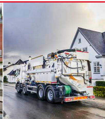
Bucher SuperRecycler CR140 3,079 UK gal (14 m 3 ) tank. 14.5 psi overpressure. Extra compressor, movable partition and 5-step continuous recycling system.
