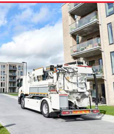
Bucher Recycler CR60 1,319 UK gal (6 m 3 ) tank. 7.2 psi overpressure approved. Movable partition and 5-step continuous recycling system.
