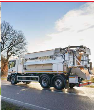
Bucher Recycler CR120 2,639 UK gal (12 m 3 ) tank. 14.5 psi overpressure approved. Movable partition and 5-step continuous recycling system.
