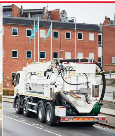
Bucher Recycler CR140 3,079 UK gal (14 m 3 ) tank. 14.5 psi overpressure approved. Movable partition and 5-step continuous recycling system.
