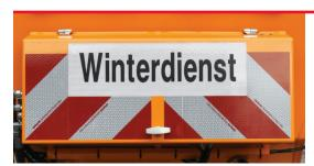
Winter maintenance and warning marks (optional) Retroreflective material according to DIN 30710.
