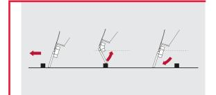
Scraping edge available in bi-shore neoprene, steel, Kombi or polyurethane. The insert between the steel blade and the side snowplough eliminates any vibrations and stops the blade from rotating if obstacles are encountered with automatic return to the operating position.
