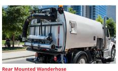
for catch basin suction and drain clearance with pendant control to aid the operator.
