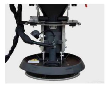
"Standard" gritting unit with 470 mm disc and all metal parts made of AISI 304 stainless steel. With asymmetry that can be adjusted to five different positions, it can spread material up to a width of 8 m. When being moved, it can be easily lifted and turned over and a sensor ensures that the plate is automatically blocked when it is lifted.
