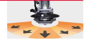
Electrical control of spreading asymmetry in 5 presettable positions
