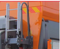
Ladder Safety ladder on RH rear side in AISI 304 stainless steel.
