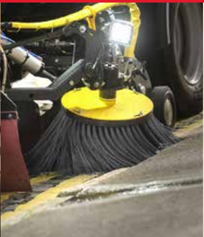
Hi-vis brush plates High visibility brush plates and hose sleeves makes it easier for the operator to see the brush position and alerts pedestrians, cyclists and other vehicles to the position of the brushes.
