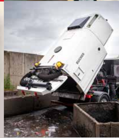
High tipping angle door And sloping hopper floor for ease of discharge.
