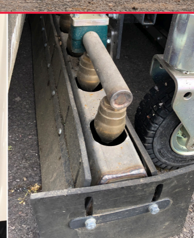
Rotating jets Optional rotating jets for high intensity cleaning in front of the rear nozzles.
