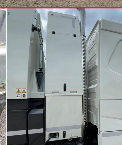
Storage locker Optional storage locker added to the 1700 l water tank provides additional storage capacity when top mounted wanderhose options are not required.
