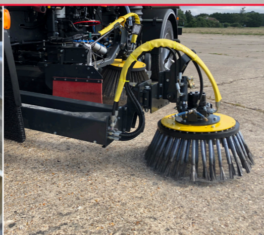
Side slide brush Optional brush behind the front wheel for increased swept width and effective weed removal without the use of chemicals.
