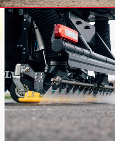
V-jet spraybar 16 High pressure v-jets to the rear nozzles as standard when rear suction and powawash are ordered together.
