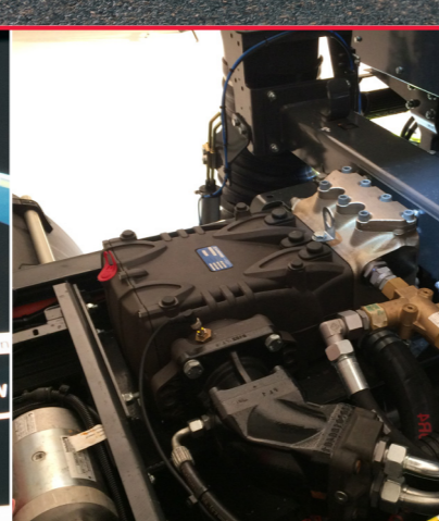
Powawash option High pressure water delivering 100 l/min @ 200 bar to a variety of spraybar options.
