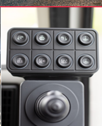
Powawash keypad Electronic water valves with in cab control for Powawash options.
