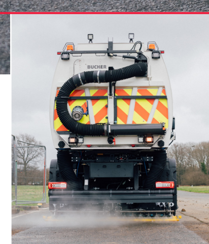
Rear suction nozzle option Full width nozzles for high performance pick up ideally suited for deep cleaning and road construction.
