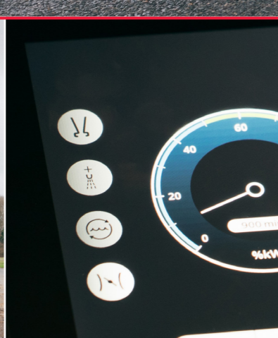
Rear nozzle operation Touchscreen operation from the JVM with separate selection for low pressure water.
