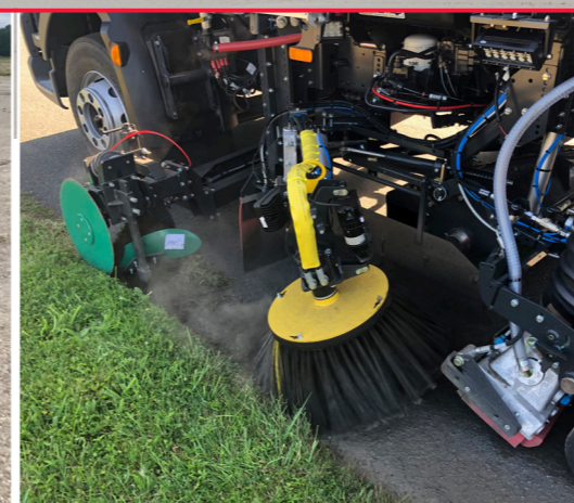
Disc coulters option Provides the ability to cut back turf ingress on non-kerbed roads leaving a clean cut edge to verges.
