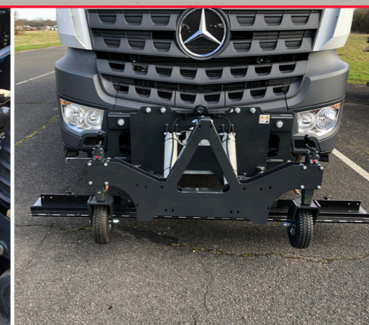
Front mounted magnet Option for the collection and removal of ferrous material in airport and industrial cleansing applications.
