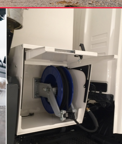
1700 litre water tank Large auxiliary stainless steel water tank with integral storage locker and high pressure hose reel and lance.
