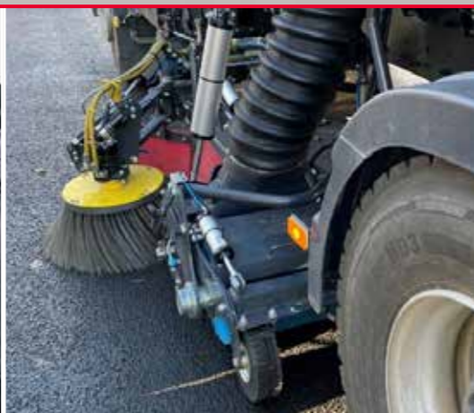
200mm BroomVak side slide Allows an additional 200mm side sliding of the nozzle and channel brush for extended swept width.
