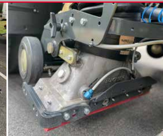
Heavy duty nozzle For aggressive environments. Offers higher grade industrial wheels, bumper and nozzle brace.
