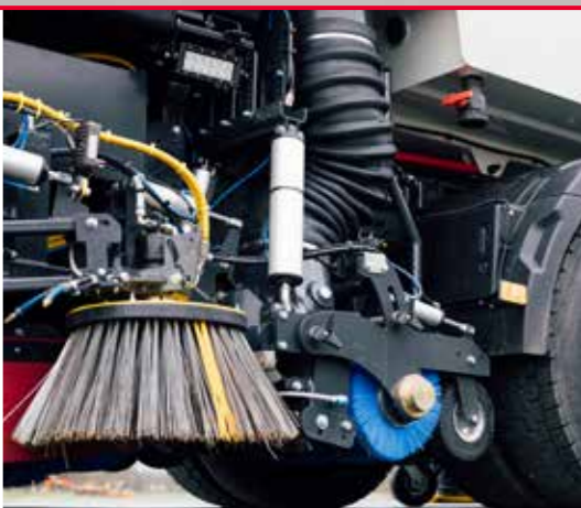
Broomvak sweepgear For high speed pick-up. Also allows pick up at reduced fan power.
