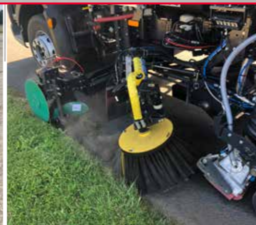
Disc coulter option Provides the ability to cut back turf ingress on non-kerbed roads leaving a clean cut edge to verges.
