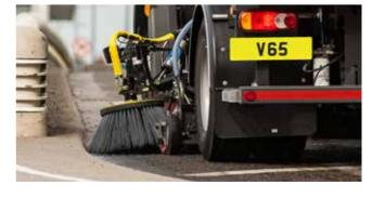
Rotatilt option adjusts the angle of the channel brush from the cab to clean crevasses and cambered roads.
