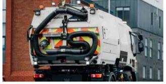
A long seven metre reach Littasnatch with air operated gate designed for the collection of lightweight debris in hard to reach places.
