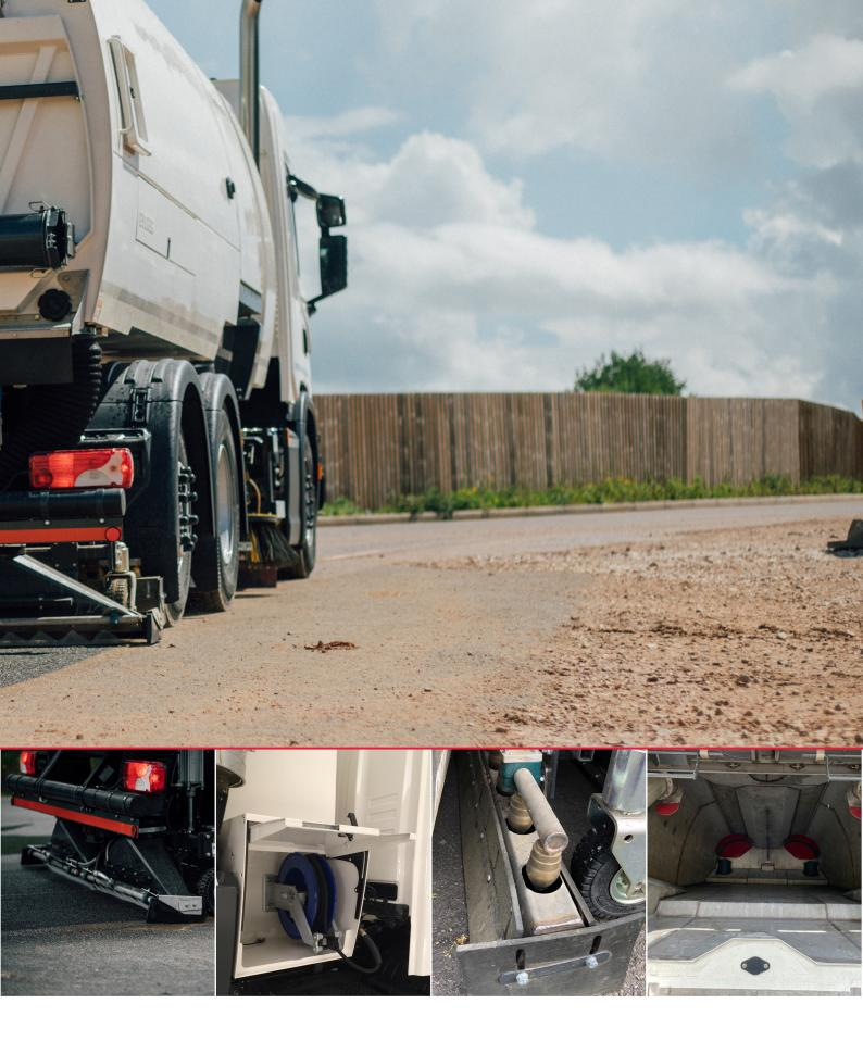
V-jet spraybar 20 High pressure v-jets to the rear nozzles as standard when rear suction and pow-awash are ordered together.
