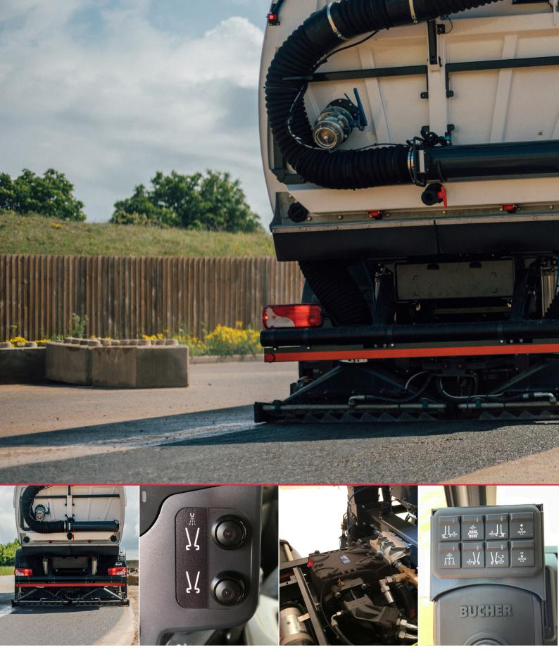
Rear suction nozzle option Full width nozzles for high performance pick up ideally suited for highways and road construction.
