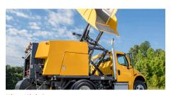
**Ultra High Dump** providing an additional 18 inch tip height ideally suited to transferring debris into a tipper truck.
