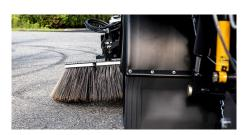
**Rotatilt** allows in-cab adjustment of the gutter brooms to suit the changing profile of the road.
