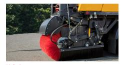
Main Broom hydraulically driven polypropylene main broom with floating trailing arms.
