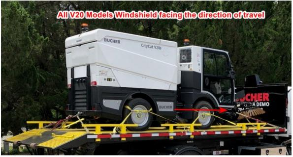
Note; Any Damage or Violation of BMNA Loaned Equipment will the responsibility of the Borrower. All Damage Cost will be Invoiced at time of repair. Note; BMNA requires ALL Tire Straps and Chain Binders be used during transportation.
