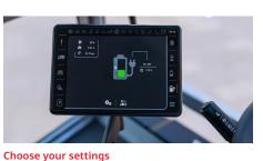
The CSense display (10.1 inch touch display) with intuitive design for extended functions, central overview of all settings and visual diagnostic system. The displayed vehicle set-up can be individually chosen by the driver.
