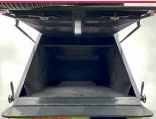
Hopper 1.8 m 3 , stainless-steel
