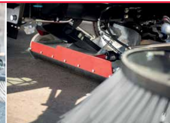
Suction intake with leaf flap
