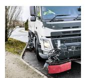
Side sliding brush unit Sweep at a distance by extending the brush and suction nozzle.
