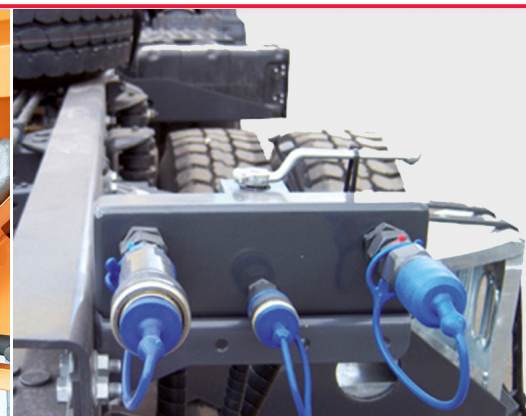
Hydraulic drive Driven by the vehicle's hydraulic system and compliant with the EN15431 European standard.
