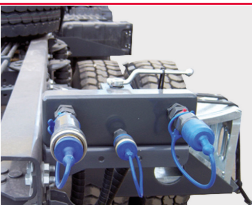
Hydraulic drive By means of the hydraulic and pneumatic system of the carrier vehicle of the drop-proof quick coupling type with rest protection included.
