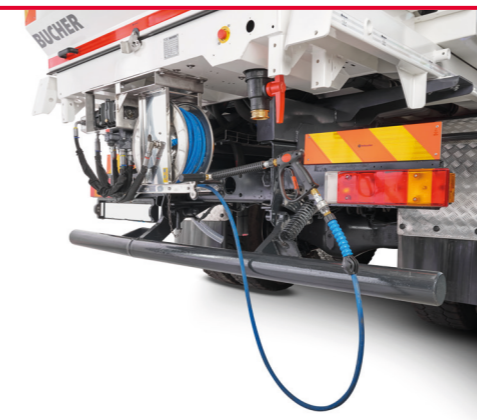
Stainless steel hose reel Equipped with hose 18 with a length of 30 meters and automatic winding. It provides a pressure of 7 bar. A high-pressure hose reel with 180 bar pressure at 15 liters per minute is available as an option.
