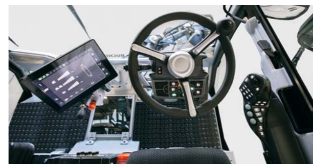
Cabin Walk through cab with clear side vision and big wind-screen. Easy reach/use control panels positioned to the front and side of the operator.
