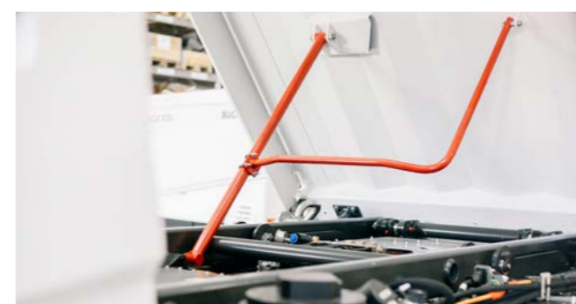
Operator safety Automatically engaged mechanical hi-vis body prop.
