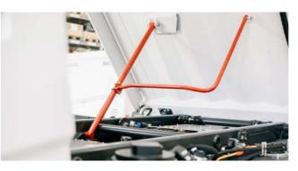
**Operator safety** Automatically engaged mechanical hi-vis body prop.
