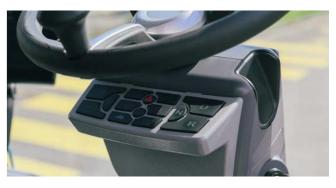
**Control panel on the steering column** The control panel contains all driving relevant buttons, easily and quickly accessible. 10
