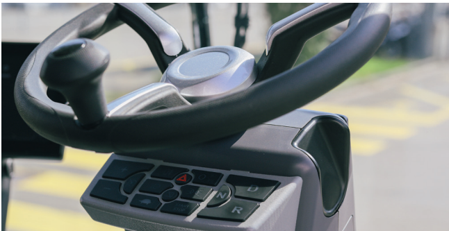
Control panel on the steering column The control panel contains all driving relevant buttons, easily and quickly accessible.
