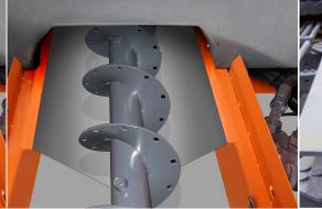
An auger with steel variable pitch coils.
