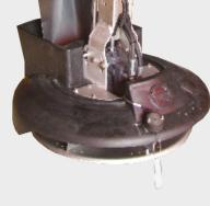
Salt sensor (optional) A mechanical sensor indicating on the control panel in the driver's cab that no salt is coming out of the spreading disc.
