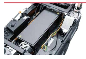
Specially designed Bucher Battery Pack with superior lifetime and no memory effect. Made with high quality automotive prismatic Li-ion NMC cells, managed through an automotive battery management system, the battery is placed in a shock, water and dust-proof case. The Bucher Battery Pack is maintenance-free and has a sophisticated repair concept for maximum safety. Due to the electric drive concept of the sweeper, maintenance and service costs in general are kept very low.
