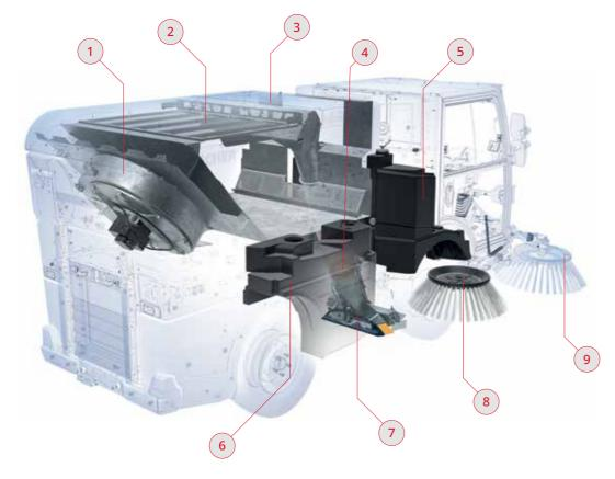
Optimised fan arrangement, with bigger, optimised blade wheels for greater efficiency
