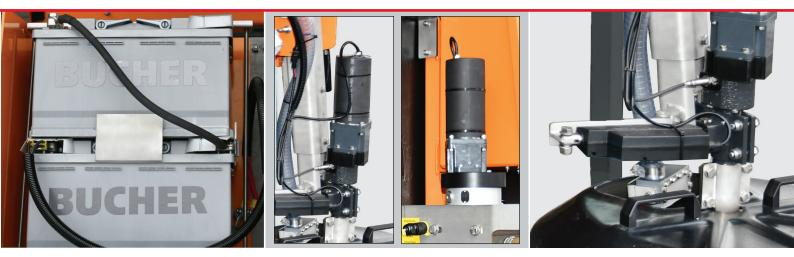
Battery buffer system Battery buffer system enables charging through vehicle recuperation.
