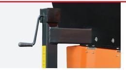
Mechanical parking system with hand crank for unloaded spreaders Mechanical or hydraulic parking systems for the loaded spreader are also available as an option.
