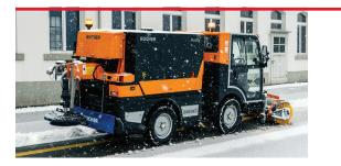
The hopper is made of high-strength HDPE (high polyethylene) and is suitable for both winter and summer maintenance.
