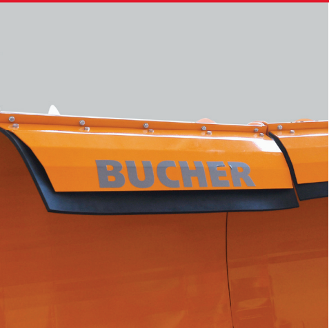
Snow dust protection (optional) Effectively protects the windscreen from snow splashes.
