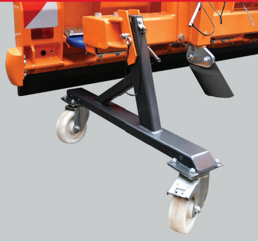
Parking device with wheels (optional) For easy transport and parking of the plough.
