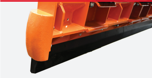
Curbstone protectors Prevent damage to the plough in case of side collisions.
