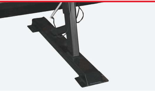
Parking support For safe parking of the snow plough.
