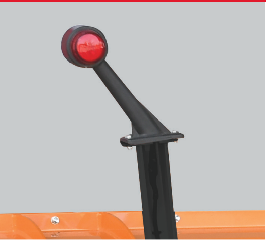
LED plough limitation lights (optional) Resistant to vibrations and external influences.
