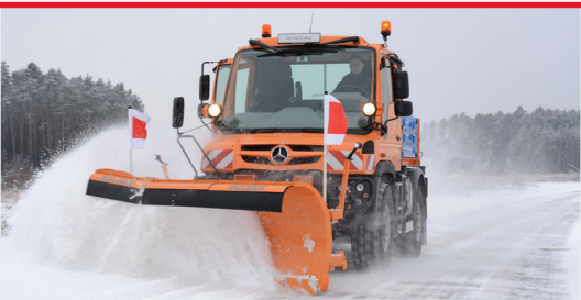
Heightened end-blade The specially shaped blade in conjunction with the heightened end-blad allows a large throwing range of the snow.
