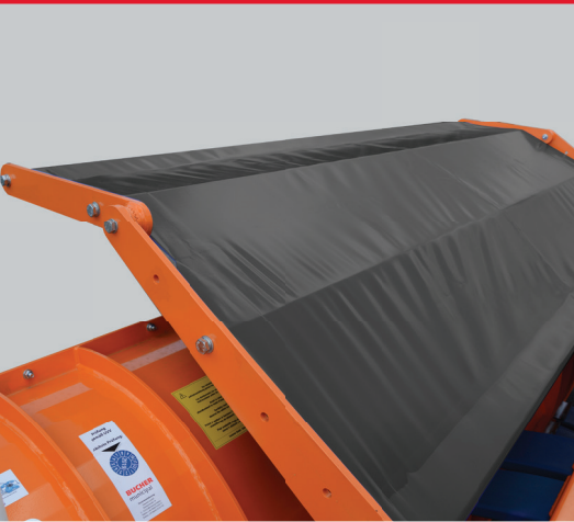
Snow guiding cover (optional) Directs snow under the vehicle to ensure a clear view for the driver.
