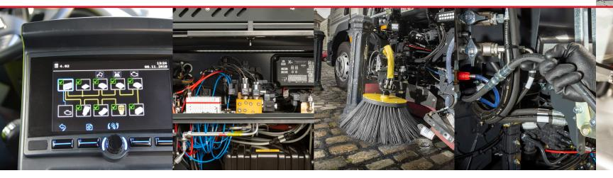
JVM system with 7" color screen provides fault diagnosis and operational feedback for the sweeper including engine codes.
