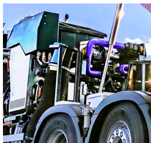
Stage V engine w. high-capacity fan High performance & payload. Low fuel consumption and noise level.
