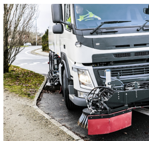
Side sliding brush unit Sweep at a distance by extending the brush and suction nozzle.
