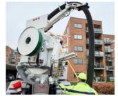
**Double telescopic arm** Reach longer and operate with less disturbance for passersby.
