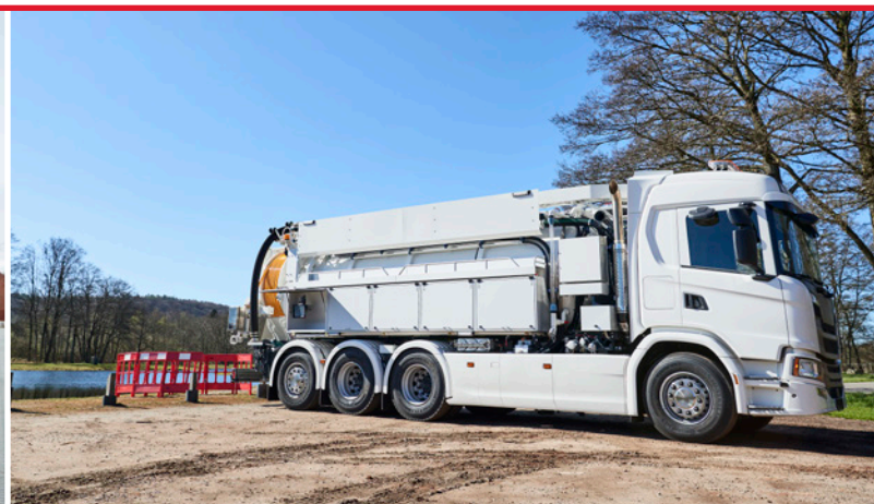
Bucher Recycler CR140 14 m 3 tank approved for 1 bar overpressure with a movable partition and 5-step continuous recycling system.
