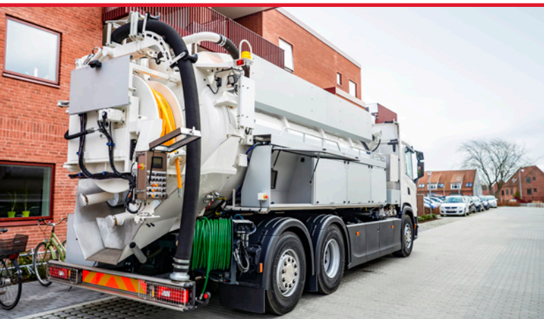
Bucher Recycler CR120 12 m 3 tank approved for 1 bar overpressure with a movable partition and 5-step continuous recycling system.
