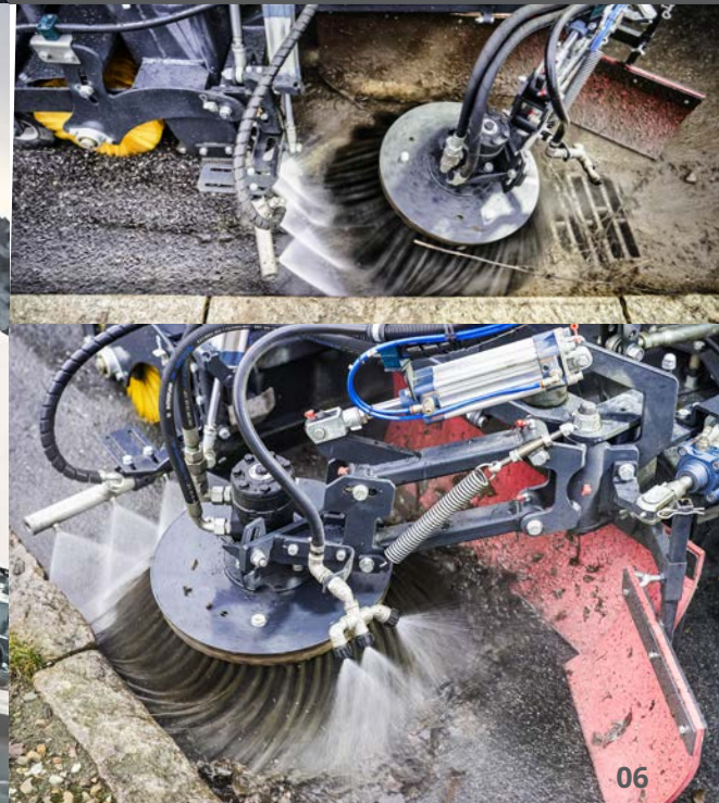
Bottom Channel brush spray bar. Channel brush spray jet cleans right into the kerb edge
