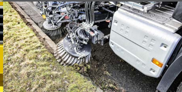
Bottom 1100mm diameter side sliding front brush
