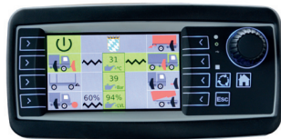
Wachendorf hydraulic terminal (optional) Wachendorf type OPUS A3S for visualisation and control of the Ecomatic hydraulic system in conjunction with one or more joysticks.
