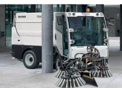
Articulated steering – maximum manoeuvrability Another advantage of articulated steering is increased manoeuvrability. With this system, the suction nozzle always faces in the direction of travel, giving a clean sweep without leaving unsightly dirt streaks behind.
