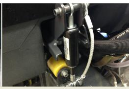
Spring struts suspension (optional) Combined spring struts are available on request. They reduce vibrations in the cab by 30 percent and thus offer maximum driving comfort.
