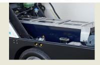
High capacity battery Pack The exceptionally robust and maintenance - free design provides a long service life and due to the liquid cooling and heating a minimized battery aging.
