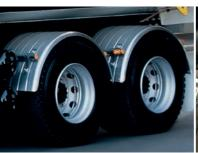
Aluminium/stainless steel mudguards Improved aesthetics and durability compared with standard plastic
