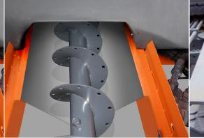
An auger with steel variable pitch coils.
