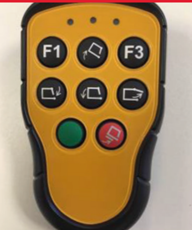
Radio controlled pendant Wireless pendant for hopper opening and tipping and wide sweep brush adjustments.
