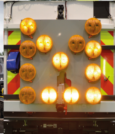
LP13 signboard An LP13 Signboard can be installed for highways contracts.
