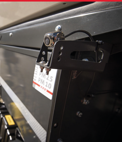
Offside camera Offside road view, providing additional vision for potential blind spot.
