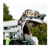
Automatic end cover Upwards opening for easy tank inspection, maintenance & emptying.
