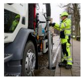
**Boom** Manually operated boom with 300° rotation.
