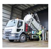
**Tipping tank** Single, front mounted, multistage tip cylinder.
