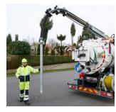
Hydraulically operated boom with 300º rotation, telescope extension, jetting pipe, and sludge breaker.
