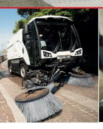
Third brush option A demountable 3rd brusharm extends the swept width by 30% to 3450mm. Control panel The palm-rest control enables operators to control the sweeping functions of the machine.
