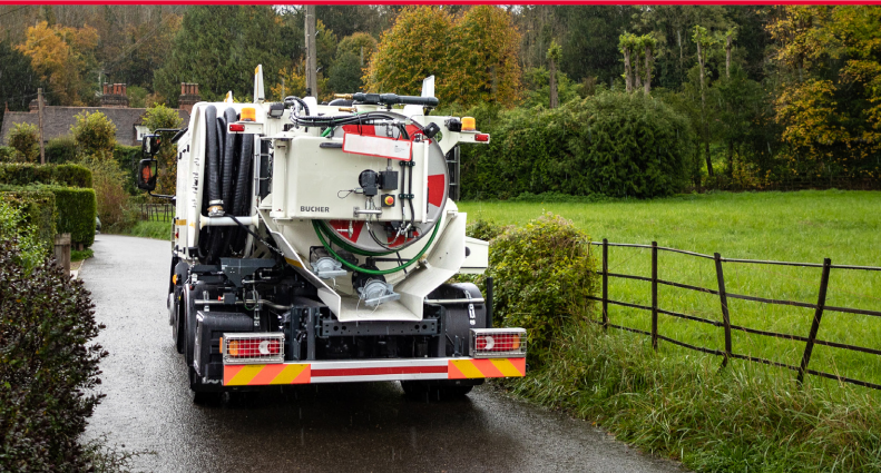
Bucher CityFlex C40 4 m 3 tank approved for 0.5 bar overpressure and a movable partition that keeps water and sludge separated.
