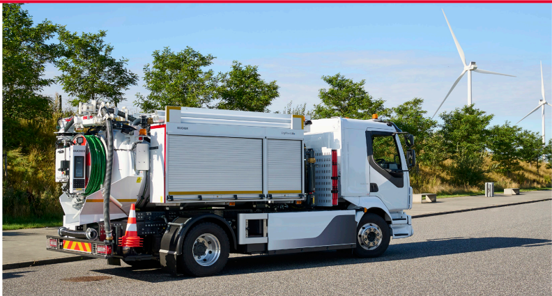
Bucher CityFlex C40e Zero exhaust emissions, low noise level and new control interface, made for operations in city centers.
